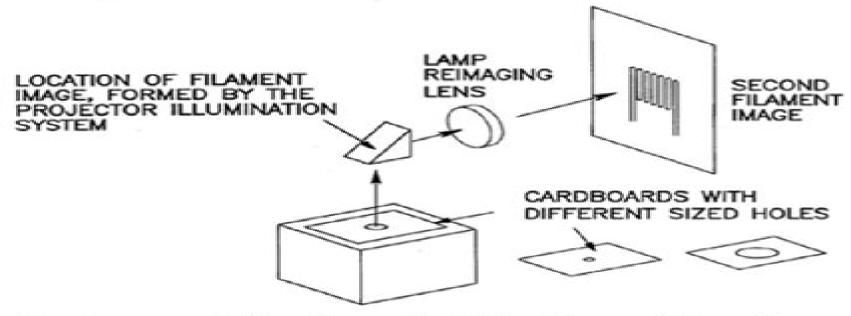
The image of the lamp that the Fresnel lens forms is not a sharp one. (The normal functioning of the projector does not require a sharp source image.)
