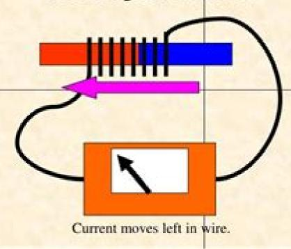
If a magnet is moved back and forth through a coil of wire, current can be made to flow through the wire. This is the idea behind electric generators and transformers.
