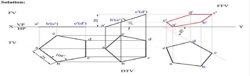
**Problem 28:** A pentagonal lamina having edges 25mm is placed on one of its corner on HP such that the perpendicular bisector of the edge passing through the corner on which the lamina rests is inclined at 30° to HP and 45° to VP. Draw the top and front views of the lamina. **Solution:**
