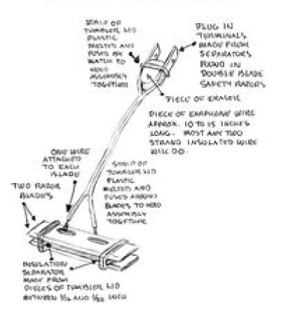
This is a design that one of my cellies mean-produced. He could assemble one in about an hour, using parts cannibalized from a couple of doubleblade safety rapors, a soft tumbler plastic lid, and double insulated wire from an earphone plug.
