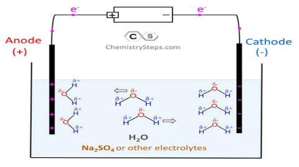
The negative end of water molecules surrounding the anode (+ in the case of electrolytic cells), and the positive end of the molecule surrounding the cathode (- in electrolytic cells):
