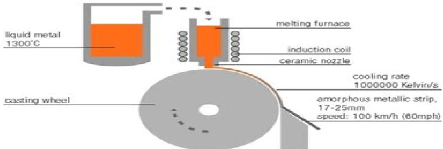
Rapid Solidification Technology allows the production of metallic ribbons in the amorphous (glassy) state. The lack of long range atomic order results in superior soft magnetic properties.
