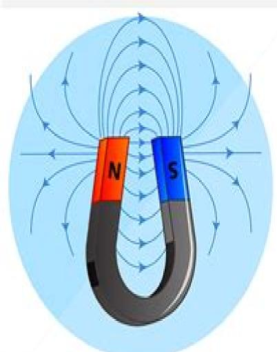
The magnetic field is an area surrounding a magnet or a moving charged particle where magnetic forces can influence other objects.
