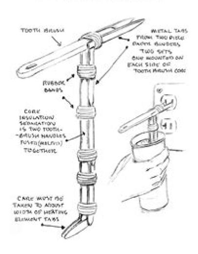
An interesting stinger design by one of my cellies. Simple and streamlined in appearance but awkward to use, since without the play offered by a flexible wire, it is necessary to hand-hold the tumbler of water while it heats.
