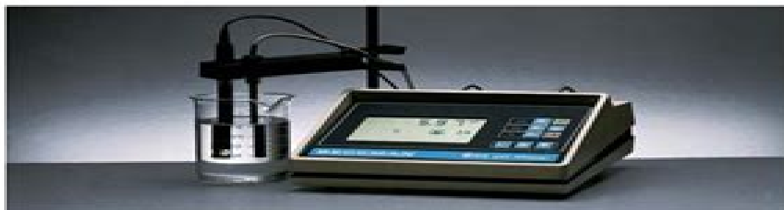
Figure 11.6 A pH meter is commonly used in the laboratory to determine the pH of a solution. Although many pH meters have scales marked with values from 1 to 14, pH values can, in fact, be less than 1 and greater than 14. The science behind the pH meter will be discussed in Chapter 13.
