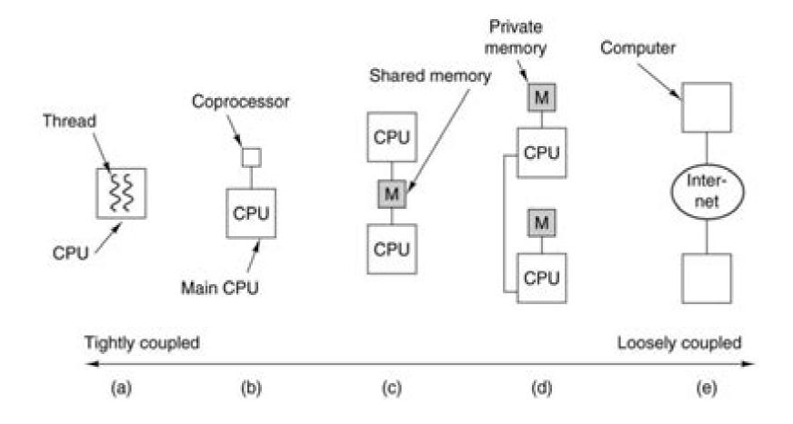
(a) On-chip parallelism.(b) A coprocessor.(c) A multiprocessor.(d) A multicomputer.(e) A grid.
