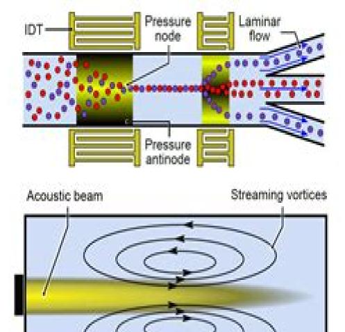
Upper figure: Particle separation in an acoustomicrofluidic device accomplished with acoustic radiation forces produced by standing waves generated in the fluid by interdigital transducers, or IDTs. Lower figure: Acoustic streaming vortices produced by the absorption of a sound beam in an enclosed fluid.
