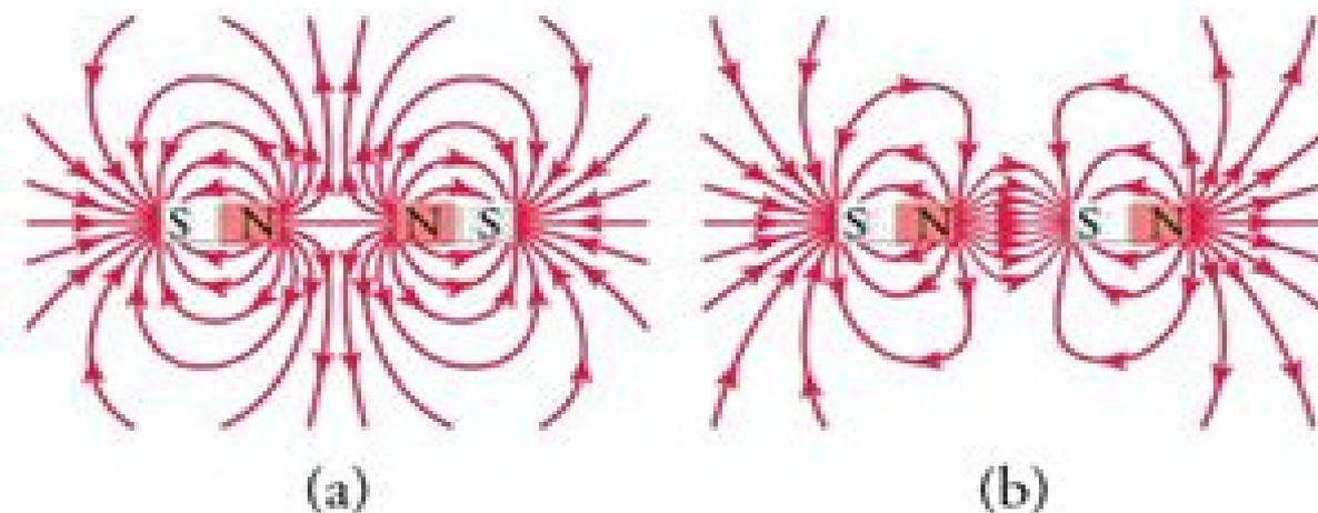
(a) When two north poles are approached together, the magnetic field lines repel each other and the two magnets experience a repulsive force. The same occurs if two south poles are approached together. (b) If opposite poles are approached together, the magnetic field lines become denser between the poles and the magnets experience an attractive force.
