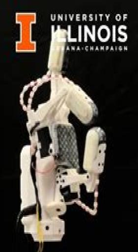
Fully 3D printable Robot Hand and Soft Tactile Sensor based on Air-pressure and Capacitive Proximity Sensing
