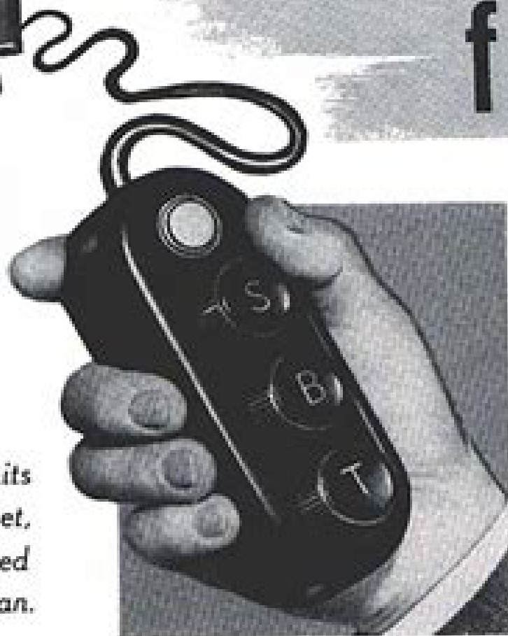
Fig. 1. The Emerson model 1158 remote-control unit shown here is capable of duplicating all of the TV set's front panel adjustments for picture and sound.
