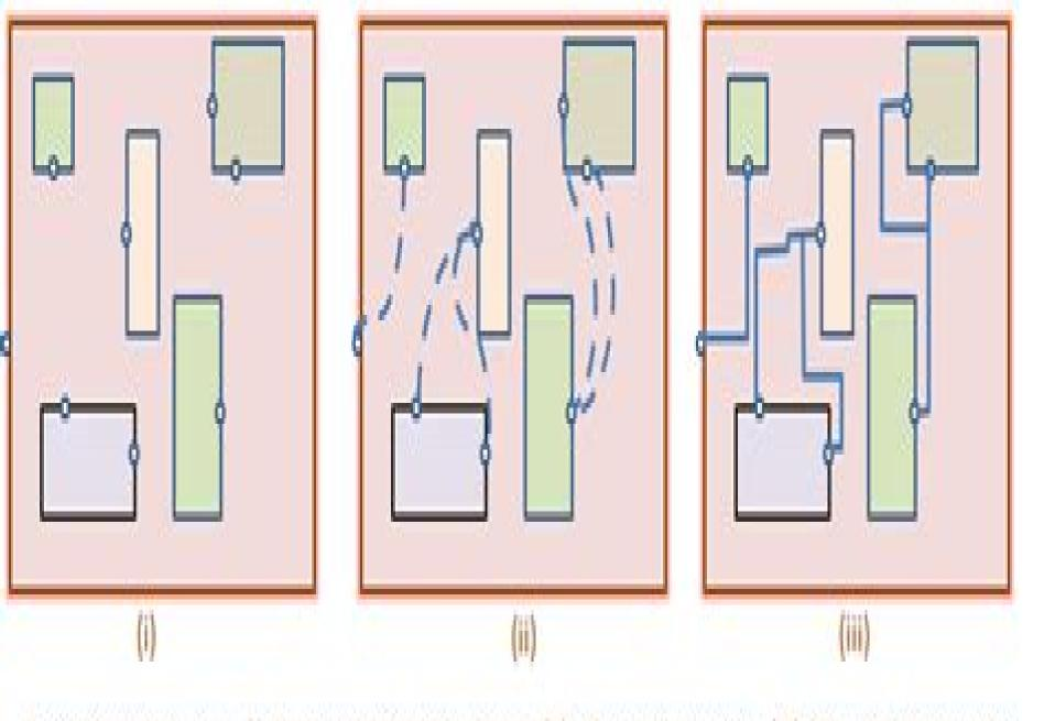
An example showing - (i) Placement of standard cells, (ii) After global routing, (iii) After detailed routing
