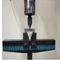
Fracture Inughness Testing
