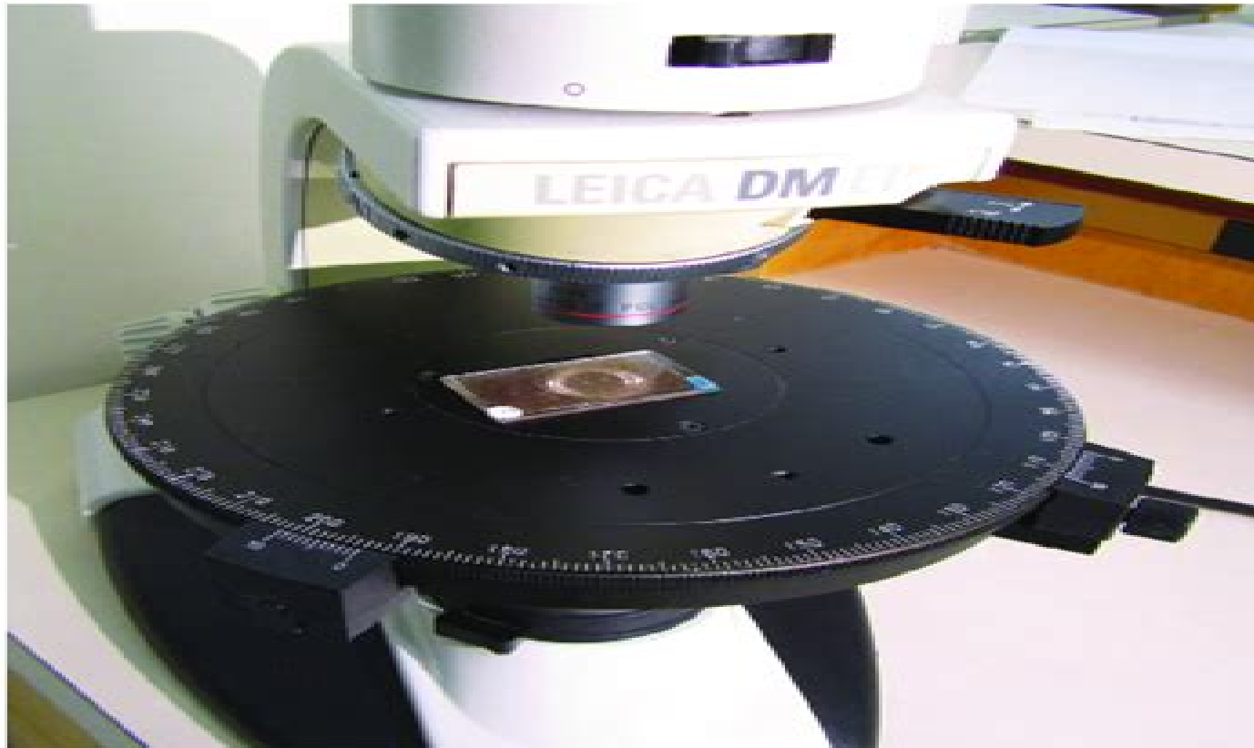
5.1 Thin section on the stage of a petrographic microscope
