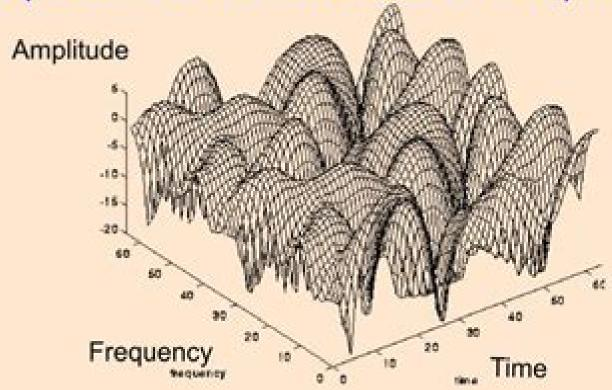
Channel Amplitude in dB versus location (= time\*velocity) and frequency
