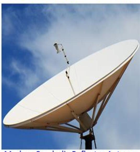
Modern Parabolic Reflector Antenna
