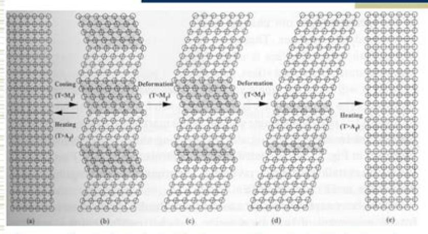
Shape memory effect mechanism, showing (a) undeformed parent crystal, (b) martensite, (c and d) deformed martensite through twin boundary movement, and (c) reversion to the parent phase after heating. From Otsuka (1998), p.37, fig. 2.11.
