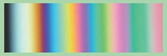
Photograph of a quartz wedge between cross-polarizers rotated 45° from extinction showing the different orders of retardation colors increasing from left to right. These colors are a true representation and not those typically seen in "colored" Michel-Levy color charts. As such these from the background image for the retardation chart from Dyar and Gunter (2020). Photograph courtesy of Michel Gunter of University of Make.
