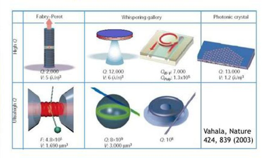
Microcavity characteristics: Quality factor Q, mode volume V
