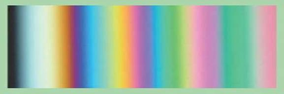
Photograph of a quartz wedge between cross-polarizers rotated 45" from extinction showing the different orders of retardation colors increasing from left to right. These colors are a true representation and not those typically seen in "colored" Michel-Levy color charts. As such these from the background image for the retardation chart from Dyar and Gunter (2020). Photograph courtesy of Mickey Gunter of University of Michel.
