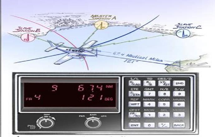
A microprocessor allows navigation to specific fixes or routes
