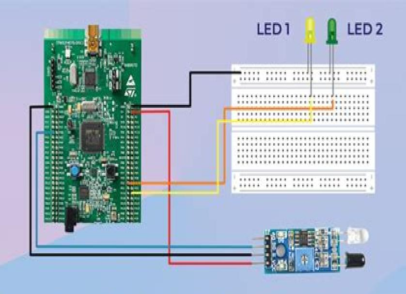
Interfacing STM32 With IR Sensor
