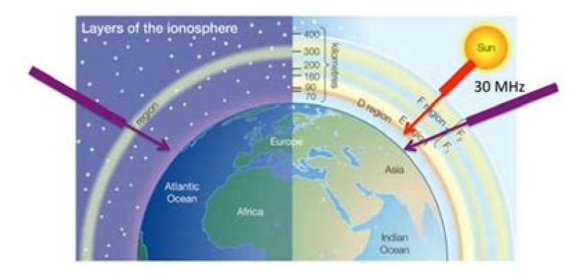
Higher ionization rate in atmosphere → higher electron density → more electrons to steal energy from radio waves → less radio wave energy at riometer site
