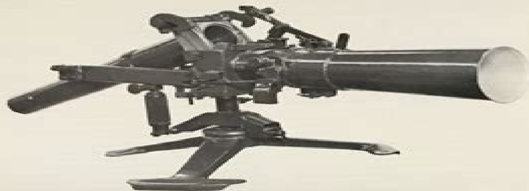
LQ 43 showing the unusual way in which the barrel dropped down and opened the breech in the same way as a shotgun to allow the gun to be loaded. (Vickers)
