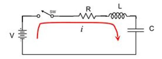
Current in an RLC circuit like shown Is governed by the equation  $V = iR + L\frac{di}{dt} + \frac{1}{C} \equiv i dt$
