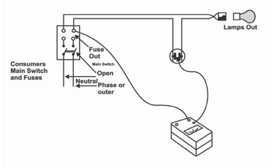
Fig 1.17 Testing for polarity of switch with circuit dead.
