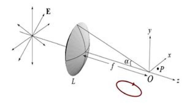
The electric field in the focal region has two components: one radial, the other longitudinal. The polarization ellipse is perpendicular to the focal plane.
