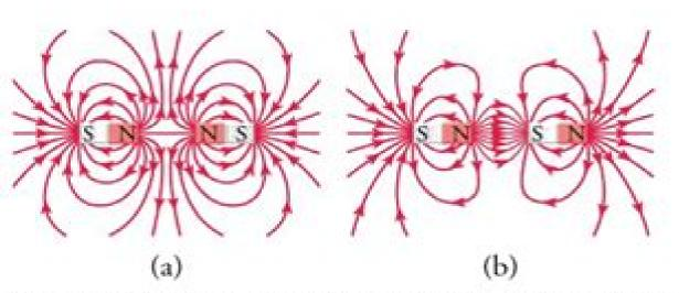
(a) When two north poles are approached together, the magnetic field lines repel each other and the two magnets experience a repulsive force. The same occurs if two south poles are approached together. (b) If opposite poles are approached together, the magnetic field lines become denser between the poles and the magnets experience an attractive force.
