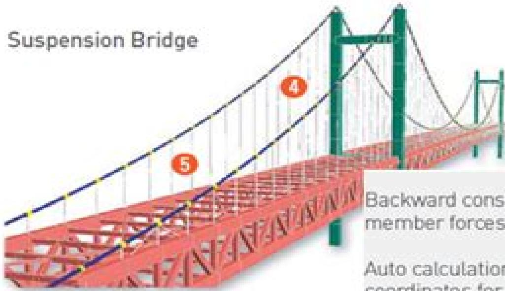
Backward construction stage analysis using internal member forces (reflecting large displacement)
