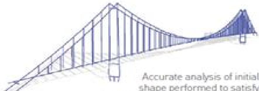
Accurate analysis of initial shape performed to satisfy the coordinates of towers and sags
