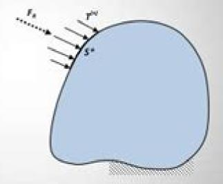
Boundary loading  $T^{eq}$  would produce detailed and characteristic effects only in the vicinity of  $S^*$ . Away from  $S^*$  the stresses would generally depend more on the resultant  $F_R$  of the tractions rather than on the exact distribution
