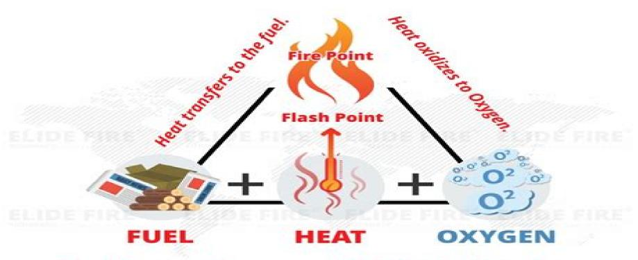
Fuel, Heat and Oxygen combined in the right mixture, Causing the Flash Point, Fire Point, and Autoignition.
