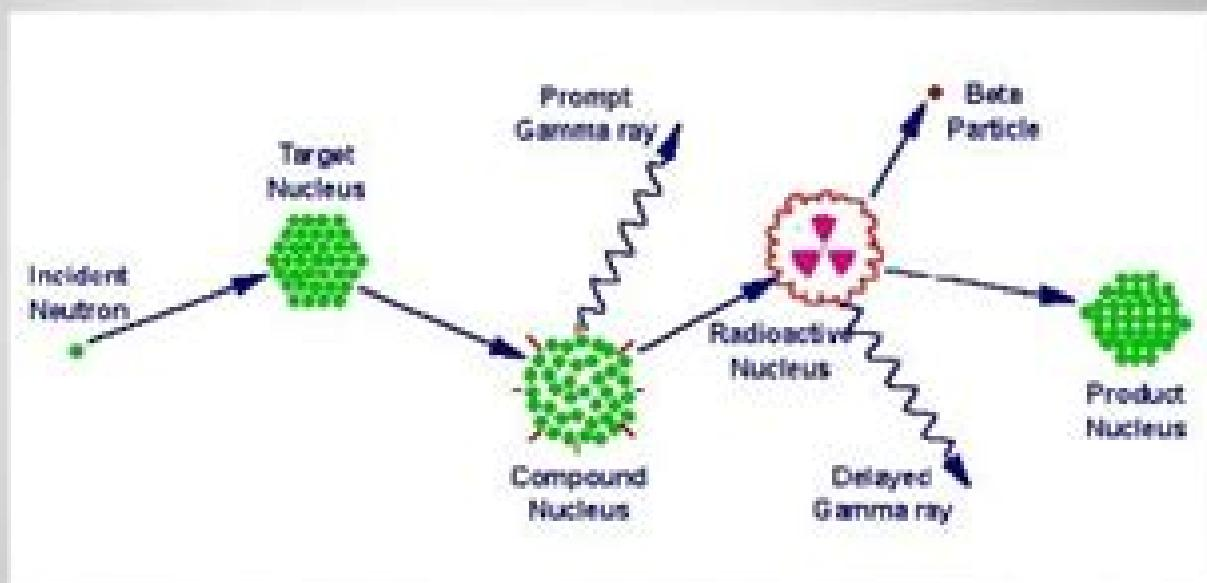
Fig. 1. Diagram illustrating the process of neutron capture by a target nucleus followed by the emission of gamma rays. The above figure is from [http://www.missouri.edu/~glascock/nna\\_over.htm](http://www.missouri.edu/~glascock/nna_over.htm)
