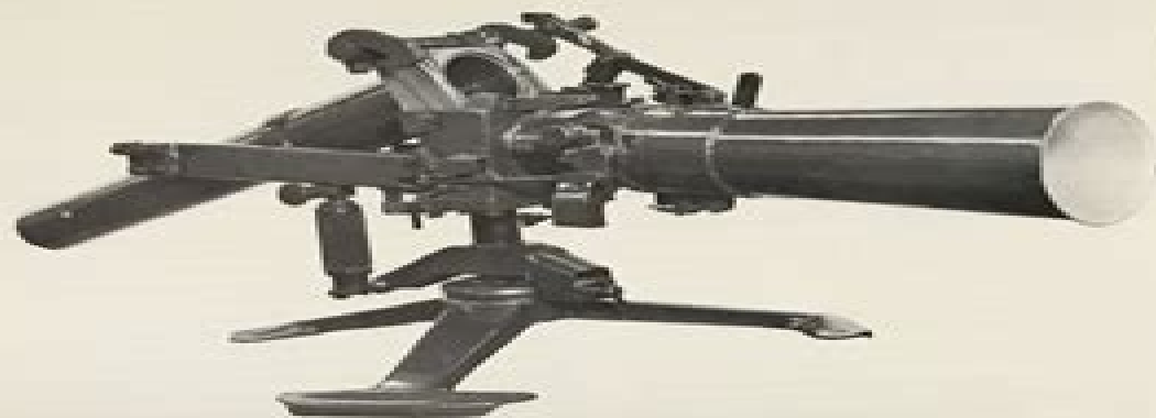
QJ 43 showing the unusual way in which the barrel dropped down and opened the breech in the same way as a shotgun to allow the gun to be loaded. (GUNS)
