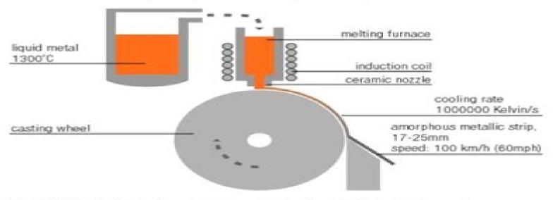
Rapid Solidification Technology allows the production of metallic ribbons in the amorphous (glassy) state. The lack of long range atomic order results in superior soft magnetic properties.
