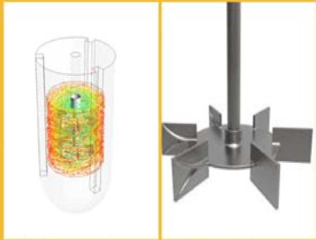
THE PRESENT PROBLEM SIMULATES FLUID MIXING IN A BIOREACTOR
