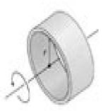
Thin ring or hollow cylinder about its axis  $I = ARR^2$
