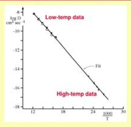
Measurement of composition profiles with high spatial resolution permits extraction of lowtemperature diffusion data because the small diffusion distances at low T are detectable by AEM X-ray microanalysis. Here Zn profiles across a 200 nm wide precipitate-free zone in Al-Zn are used to determine values of the Zn diffusivity at T = 100-200°C.
