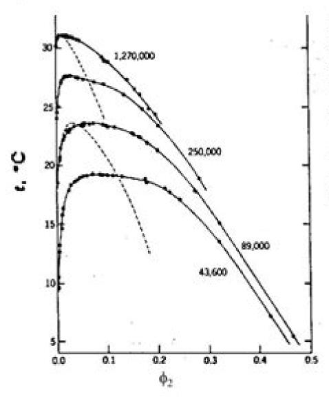
Phase diagrams for four samples of polystyrene mixed with cyclohexane plotted against the volume fraction of polystyrene. The molecular weight of each fraction is given.
