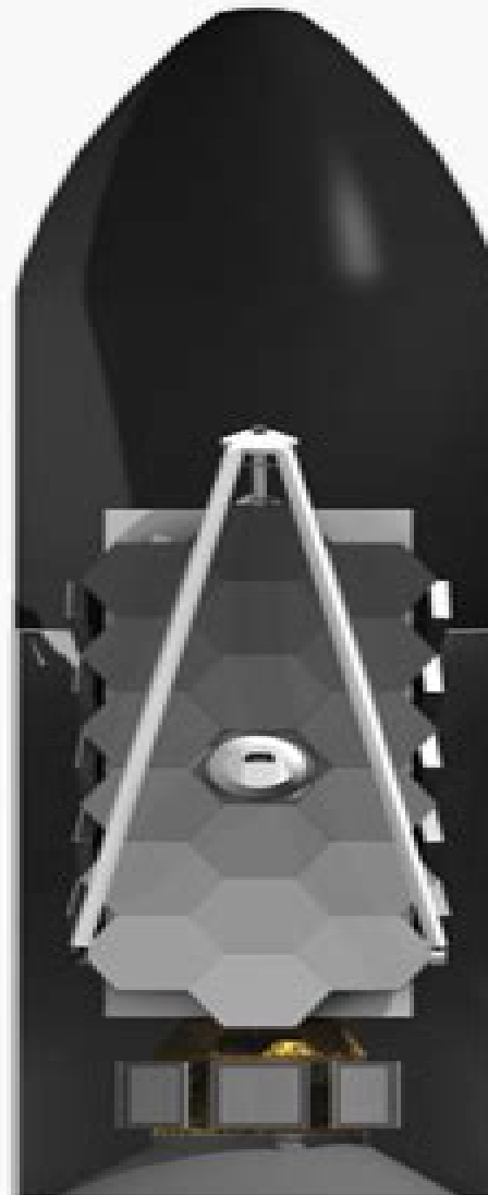
8m fairing with large aperture telescope
