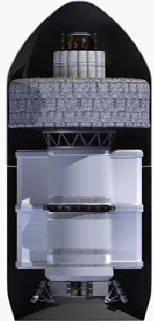
10m fairing w/notional Mars payload
