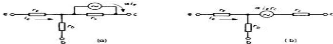
Fig. 2.11. A three-terminal active network which can be used as an equivalent circuit for a transistor (a) including a constant-current generator, and (b) a constant-voltage generator
