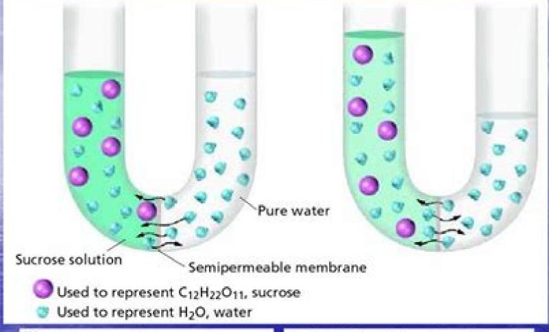
When pure water and an aqueous sucrose solution are separated by a semi-permeable membrane, the net movement of water molecules through the membrane is from the pure water side into the aqueous solution. The level of the solution rises until pressure exerted by the height of the solution equals the osmotic pressure, at which point no net movement of water molecules occurs.
