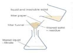
Filtration: An undissolved/insoluble solid can be separated from a solution by passing it through a piece of filter paper in a filter funnel. The solution which passes through the filter paper is called the filtrate. The solid that stays on the filter paper is called the residue. This residue should then be washed with distilled water to remove any solution between it's solid particles.
