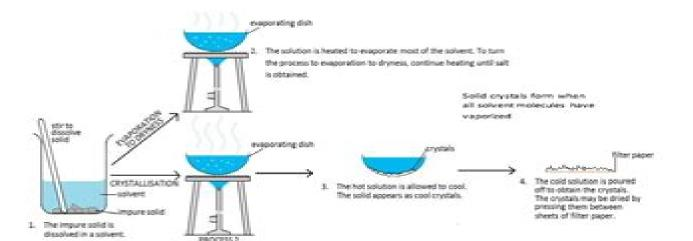
Crystallization is a process used to separate a solid in liquid misture where the solid is soluble in the solvent and dissolves in it and forms a homogeneous solution. Example: A mixture of NaCl and water.
