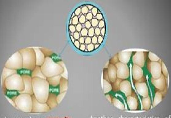
A good reservoir rock must have *porosity* in which petroleum can exist.
