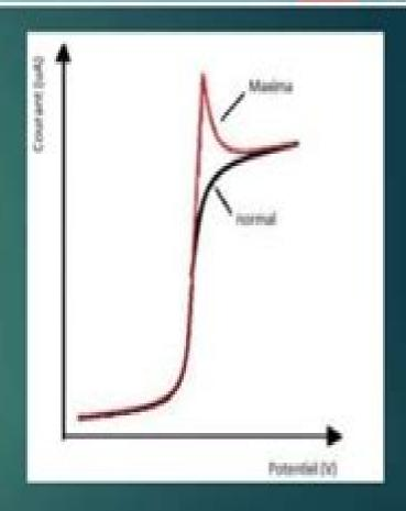
The presence of this reproducible polarographic maxima leads to error in determining half wave potential and diffusion current.
