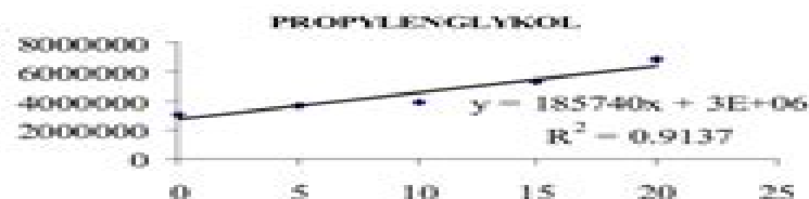
Fig. 2. Linear regression analysis shows dependence of average area on the volume of the stock reference compound mixture for 1,2-propanediol
