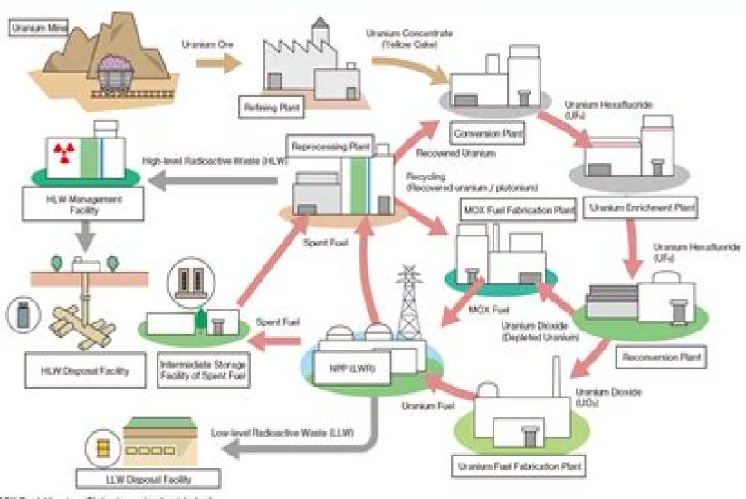
(Note) MCX Fuel: Uranium-Plutonium mixed oxide fuel
